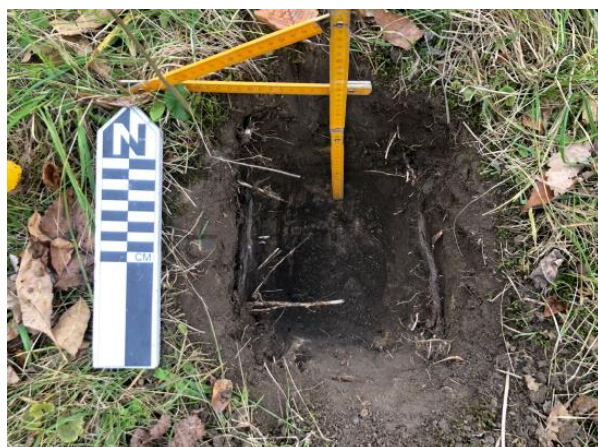
Image 5: Test pit in eastern portion of subject property, showing topsoil over clay fill.
