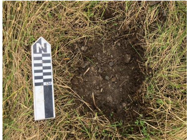
Image 4: Test pit in western portion of subject property, showing gravel road.
