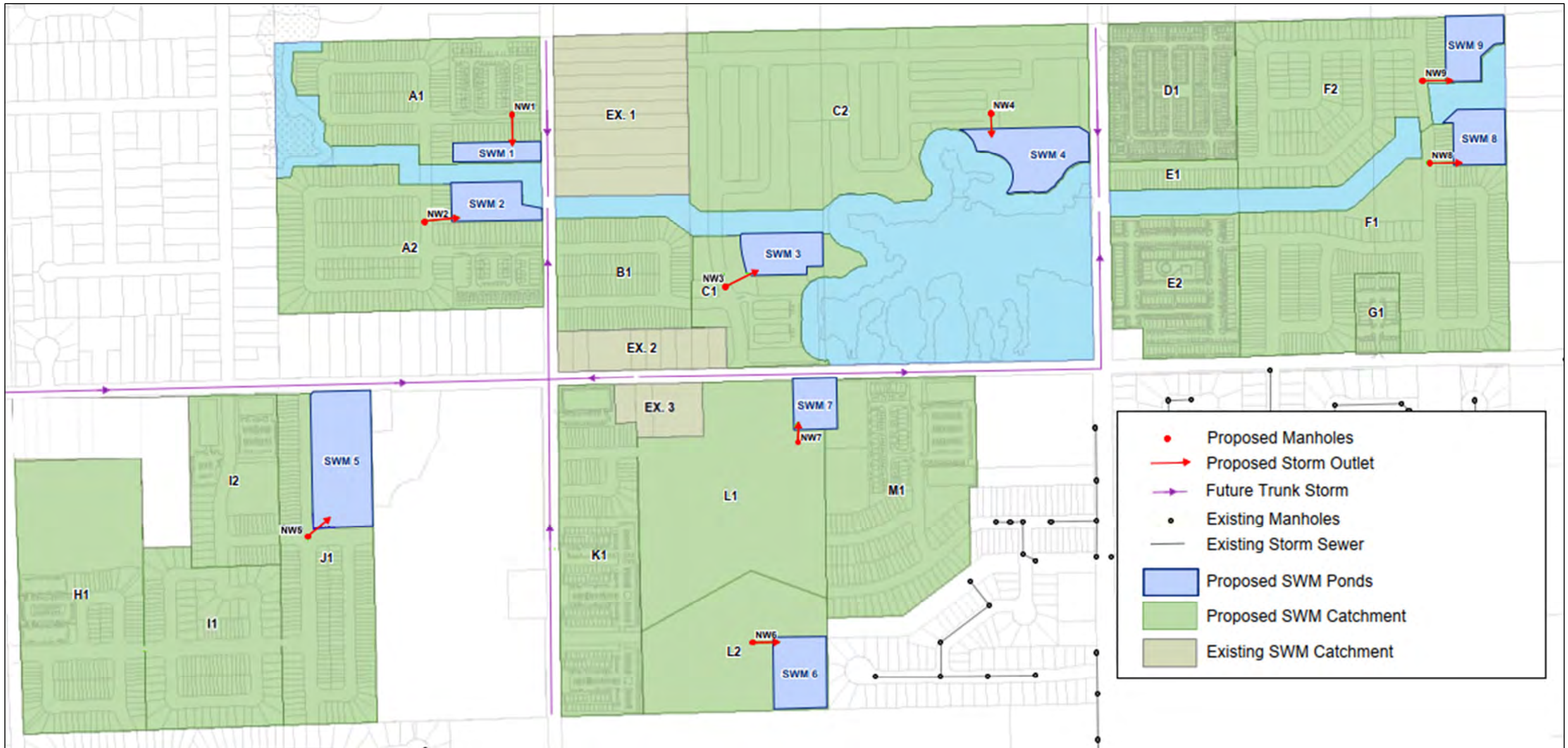
Figure 5-2: Proposed Storm System and Drainage Areas
