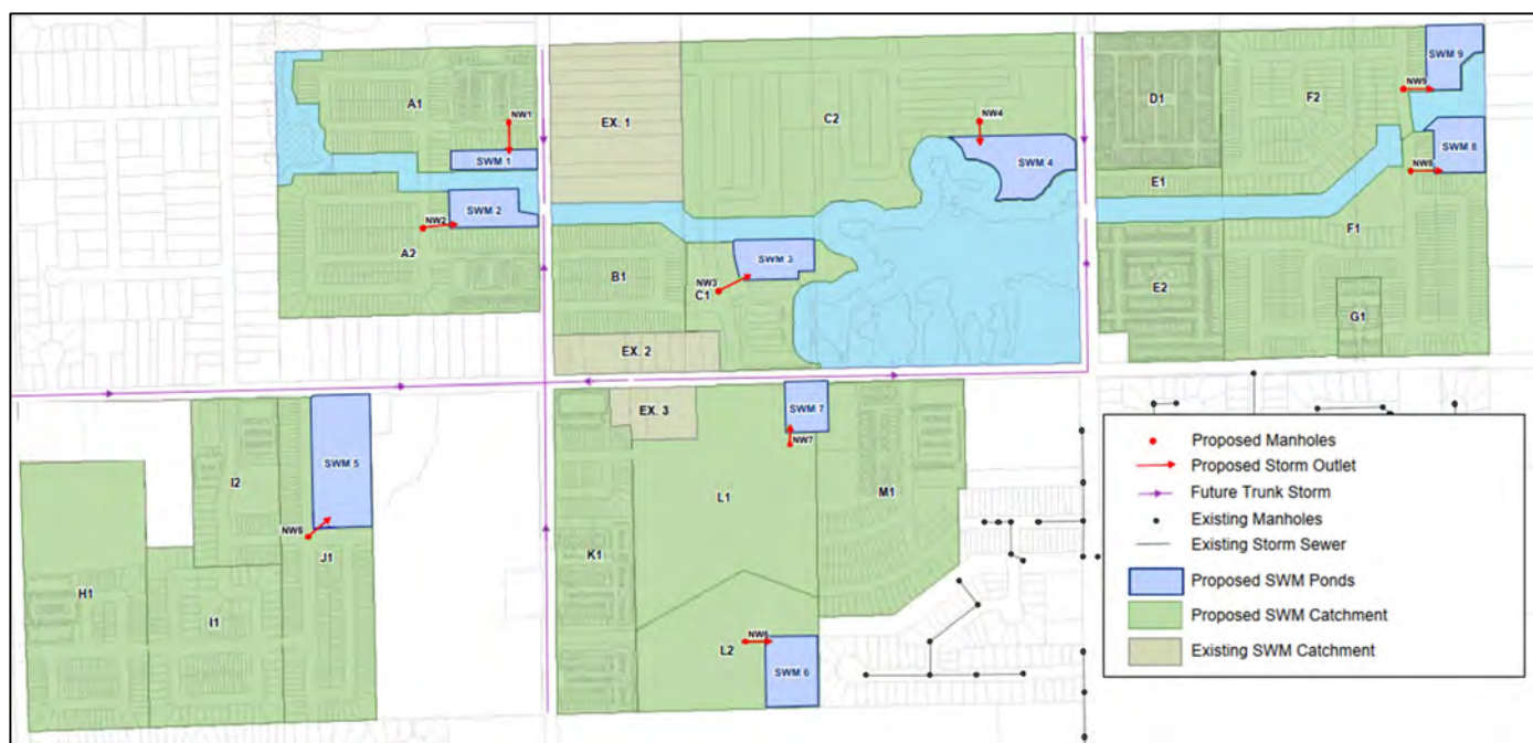
Figure 5-2: Proposed Storm System and Drainage Areas
